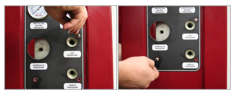
• Install new manifold onto pump frame.
