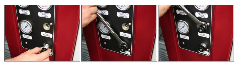
Install control knobs "Cut" and "Pierce" into respective ports on front of manifold.
