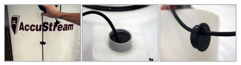
• Drop the float gauge into the tank and bring the plug end through the grey opening at the top. Attach the rubber stopper to the cord and reinsert into the grey opening. Make sure to adjust the cord to be 10" from top of tank to metal bullet.
