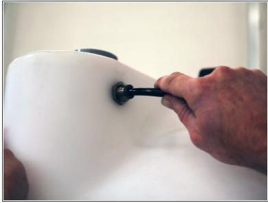
• Connect the "permeate" line to the bulkhead fitting in the water storage tank.
