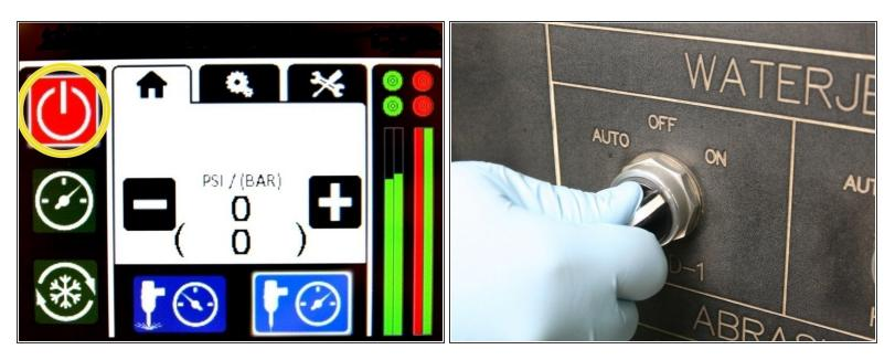
Always make sure all high-pressure water has been removed from the valve by following the machine manufacturers' safety instructions. Failure to do so can cause severe injury or death.
