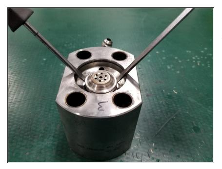
Carefully lift the check valve assembly using two flathead screwdrivers in the groove on the check valve body
