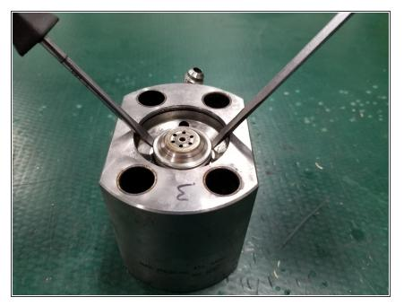
Carefully lift the check valve assembly using two flathead screwdrivers in the groove on the check valve body
