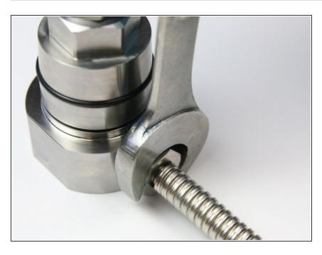
Tighten the high-pressure gland into the swivel housing with a 13/16" wrench.
