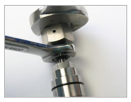
Tighten the high-pressure gland into the coupler with 1-1/16" and 5/8" wrench.
